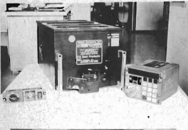
FIGURE 4. TYPICAL ARINC 561 INS GEAR
